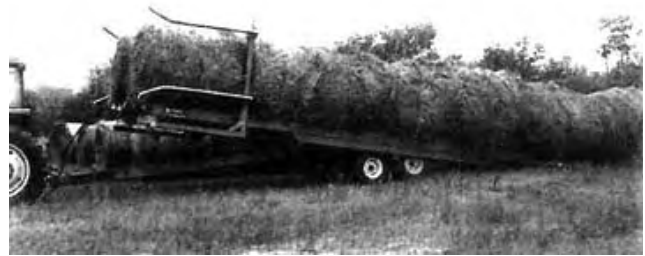
FIGURE 3. Unloading Bales from the Kingsman 217.
